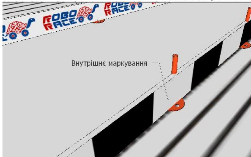
Figure 2. – An example of internal side marking of the playing field.
