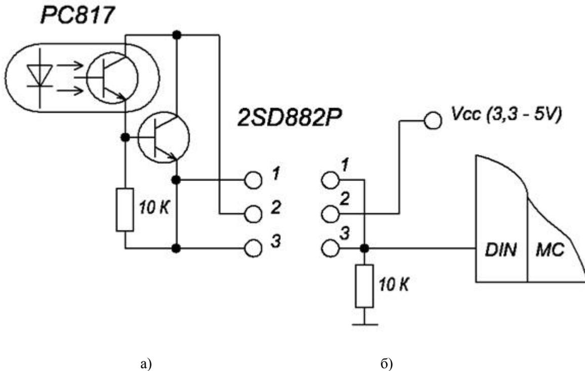
Fig.8.- The output circuit of starting device (a), recommended scheme (б).
