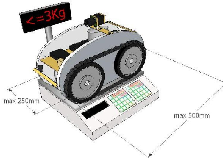
Figure 6. – The maximum dimensions and weight of the robot.
