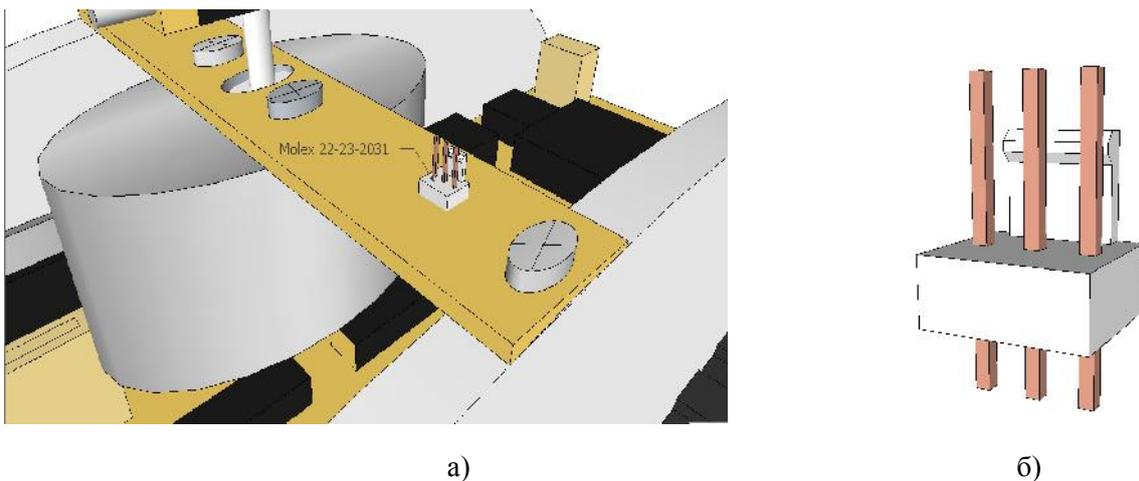
Fig.7. – Connector Molex 22-23-2031(a – example of location, б – appearance).
